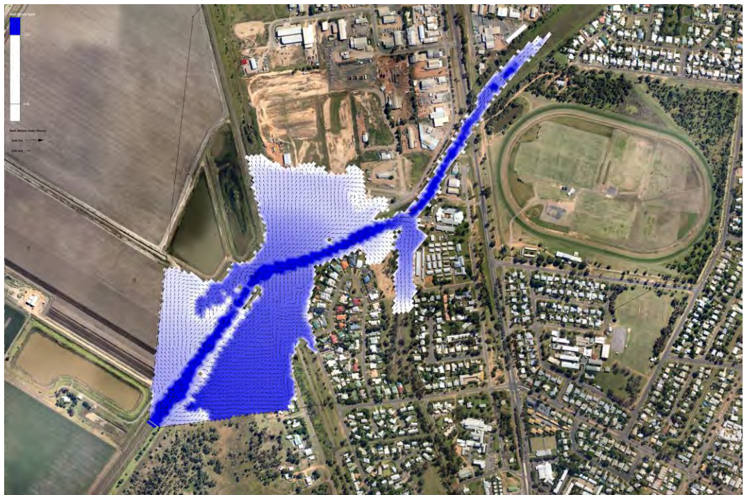
Figure 9: Modelled 100 m 3 /sec flow along LN1 drain
