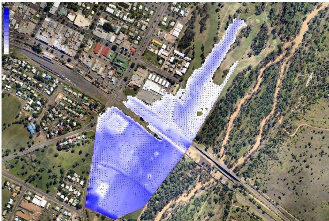
Figure 6: 500 m 3 /sec test flow including culverts under the levee
