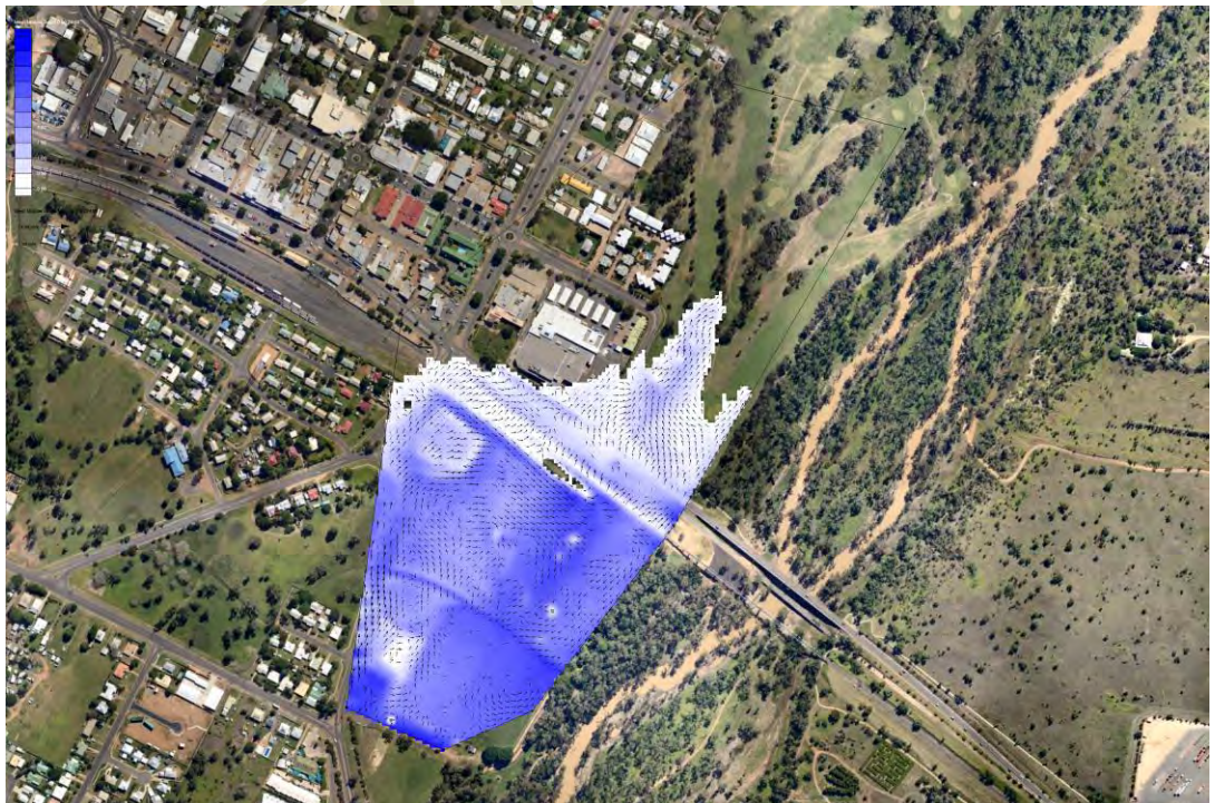
Figure 5: 500 m 3 /sec test flow with no culverts
