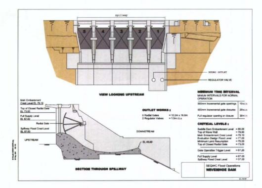
In addition to the five radial gates, the auxiliary spillway was constructed in 2005 as part of an upgrade to improve flood adequacy of this storage. The auxiliary spillway consists of a three bay fuse plug spillway at the right abutment. In association with other works constructed at the dam, this gives the dam crest flood an AEP of approximately 1 in 100,000. Another one bay fuse plug spillway may be constructed at Saddle Dam Two in the future.
