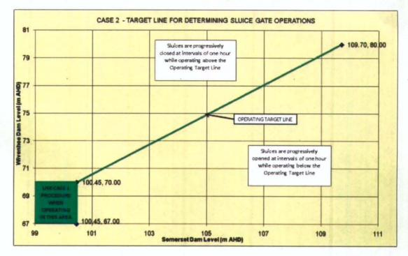
Sluices are progressively closed at one hour intervals if operating above the Operating Target Line and progressively opened at one hour intervals if operating below the Operating Target Line. The aim is always to follow the Operating Target Line as closely as possible.
