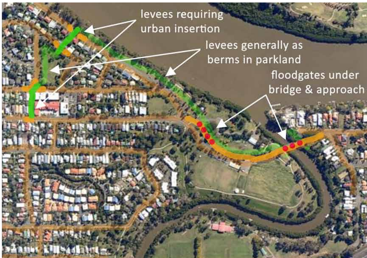
FIGURE 3: Possible Levees & Floodgates Oxley Creek (P. Skinner after Nearmap Aerial Image, Jan 14, 2011)
