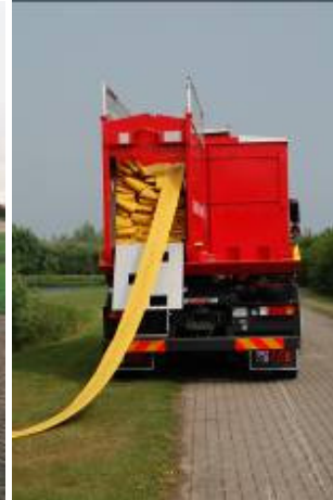
Fast hose laying
