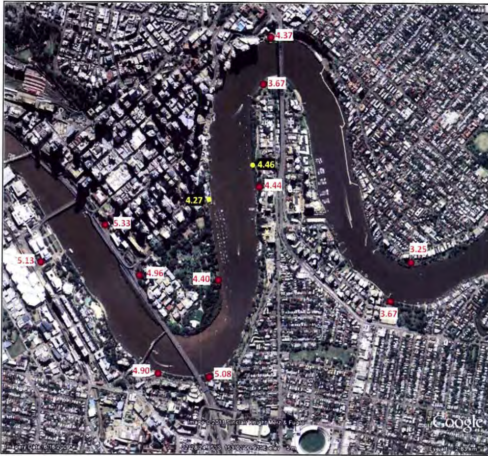
Figure 5 Peak Water Levels in Town Reach Jan 2011
