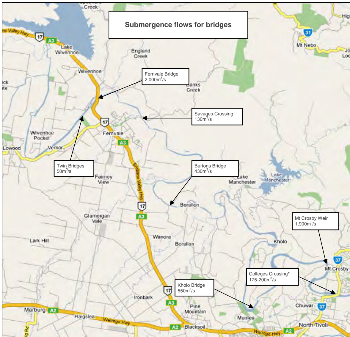
Figure 1.4.2 – Submergence flows for bridges
