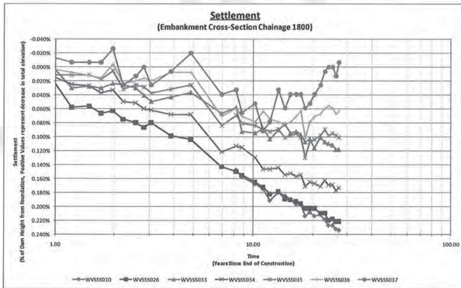
Figure 11 - Settlement of Monuments Analysed for Chainages 1,800
