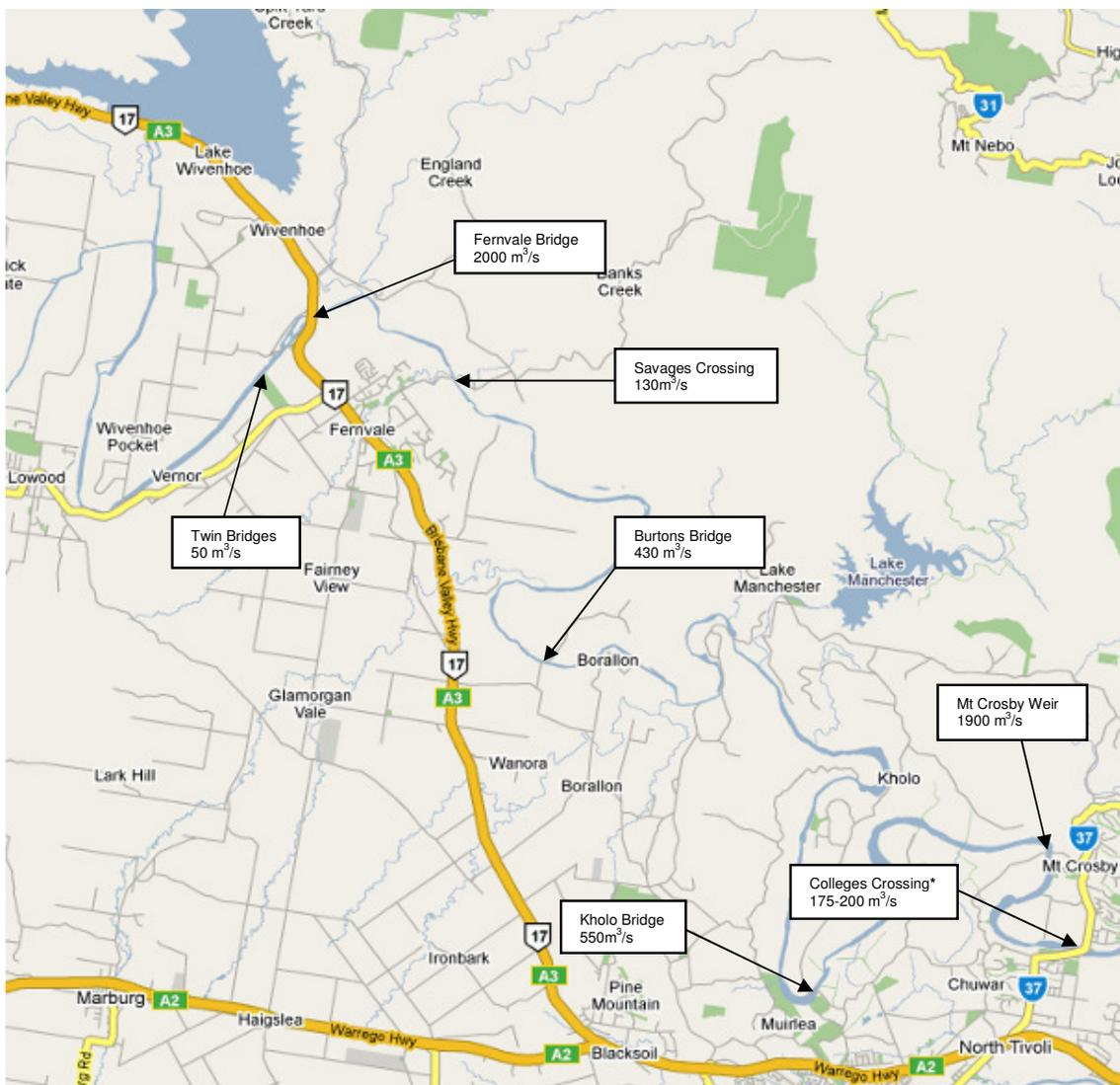
For situations where flood rains are occurring on the catchment upstream of Wivenhoe Dam and only minor rainfall is occurring downstream of the dam, releases are to be regulated to limit, as much as appropriate in the circumstances, downstream flooding.
