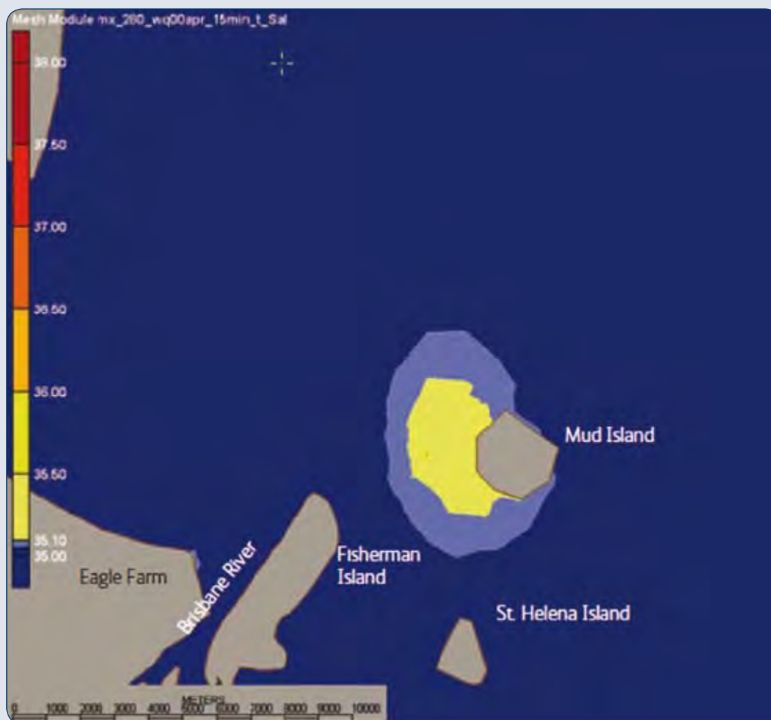
Figure 5.7 Example output from hydrodynamic modelling—median salinity contours
