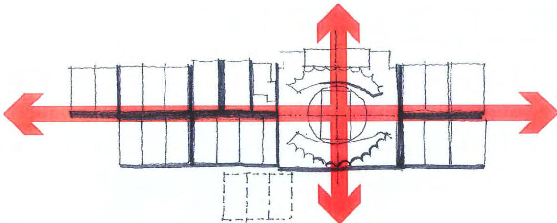
The strong east-west axis of the ladder establishes a clear differentiation between front-of-house activities and back-of-house activities. The orientation of the courts is also designed to minimise glare and wind tunnelling.
