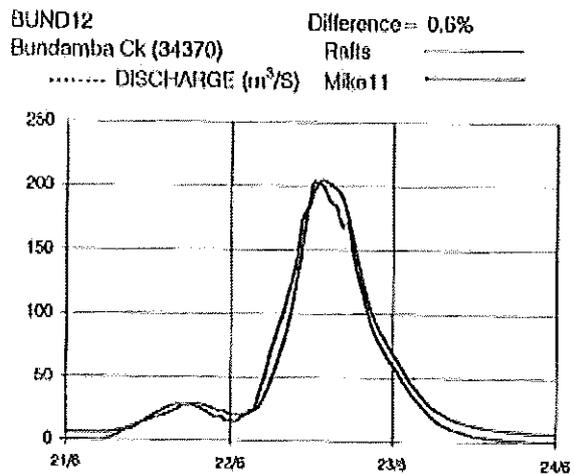
Figure E-5c - 1983 Hydrologic and Hydraulic Model Consistency
