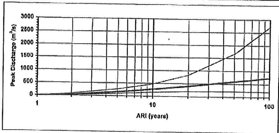
**Figure 7.6 Flood Frequency Analysis, Bremer River at David Trumpy Bridge, Ipswich shows the plotted data and fitted probability distribution for the peak stage data at David Trumpy Bridge on the Bremer River.**
