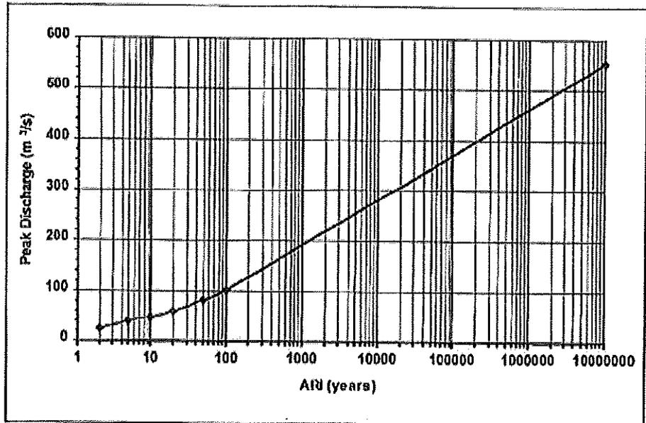
**Figure 7.15: Existing Conditions Design Peak Discharges for Sandy Creek (Chuwar) - RAFTS Node SC-OUT**
