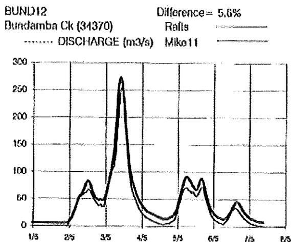
Figure E-3c 1996 Hydrologic and Hydraulic Model Calibration
