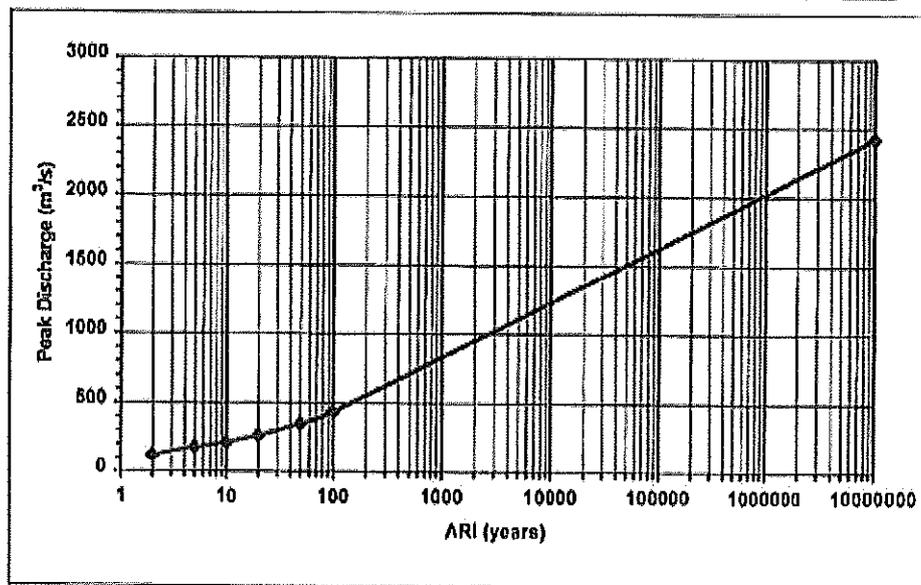
**Figure 9.10: Ultimate Conditions Peak Discharges for Six Mile Creek – RAFTS Node JINAO**
