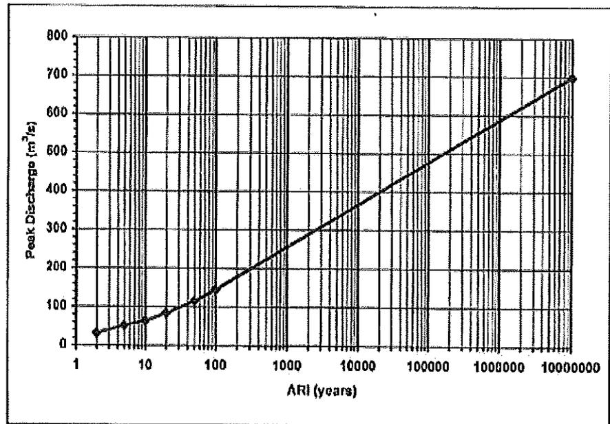
**Figure 9.9: Ultimate Conditions Peak Discharges for Bundamba Creek – RAFTS Node BUND15**
