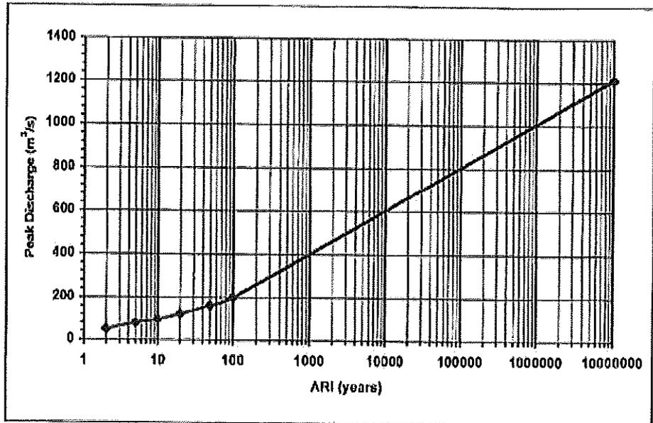
**Figure 7.13: Existing Conditions Design Peak Discharges for Ironpot Creek – RAFTS Node IP-OUT**
