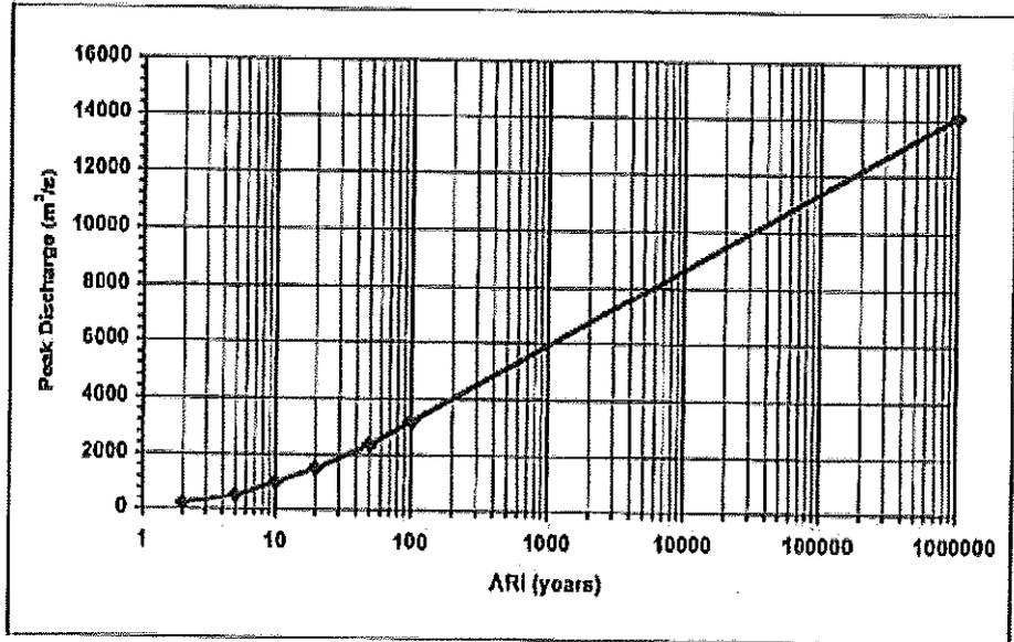
**Figure 7.11: Existing Conditions Design Peak Discharges for Purga Creek - RAFTS Node 6F**
