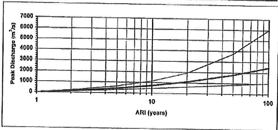
**Figure 7.5: Flood Frequency Analysis, Purga Creek at Loamside shows the plotted data and fitted probability distribution for Purga Creek with data from the 7 years of very low flows omitted.**
