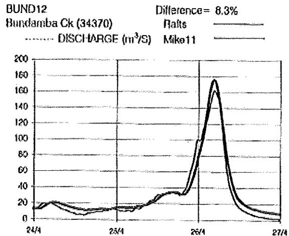
Figure E-4c - 1989 Hydrologic and Hydraulic Model Consistency
