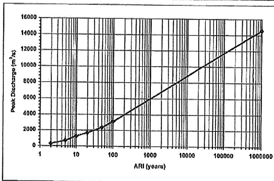
**Figure 9.3: Ultimate Conditions Peak Discharges for Warrill Creek – RAFTS Node AMB-OUT**
