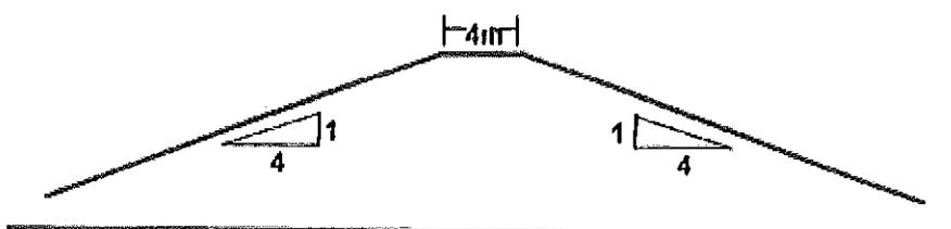
From Figure 11.4 it can be seen that if the levee is 5 metres high then the width of the levee will be 44 m wide. In residential and inner city areas this width is generally too wide and concrete levees need to be used.
