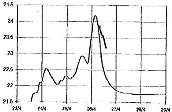
Figure D-4b Predicted & Recorded Hydrograph Comparison - April 1989
