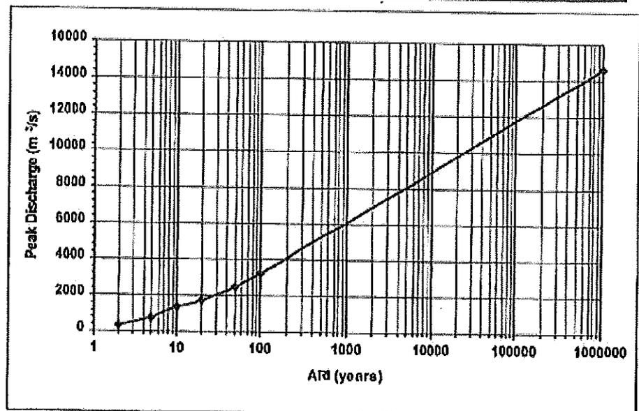
**Figure 7.10: Existing Conditions Design Peak Discharges for Warrill Creek- RAFTS Node AMB-OUT**
