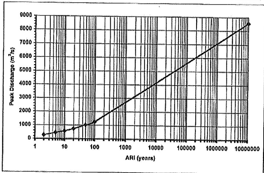
**Figure 7.12: Existing Conditions Design Peak Discharges for Deebing Creek – RAFTS Node DB-OUT**
