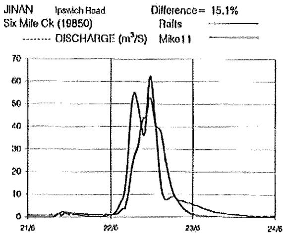
Figure E-5b - 1983 Hydrologic and Hydraulic Model Consistency
