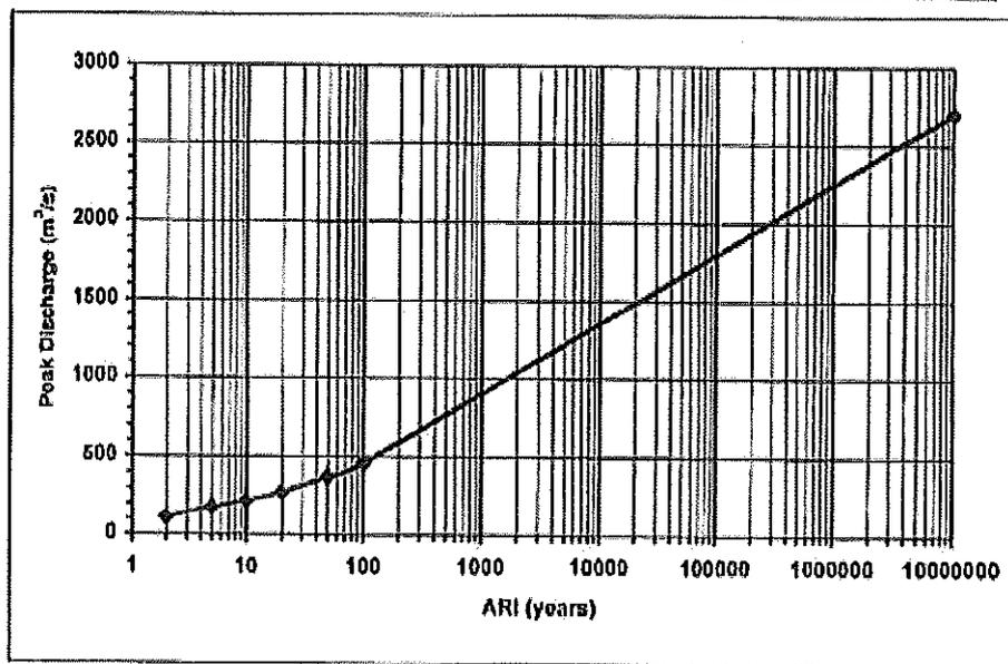
**Figure 7.17: Existing Conditions Design Peak Discharges for Six Mile Creek – RAFTS Node JINAO**
