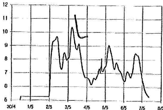
Figure D-3b Predicted & Recorded Hydrograph Comparison - May 1996
