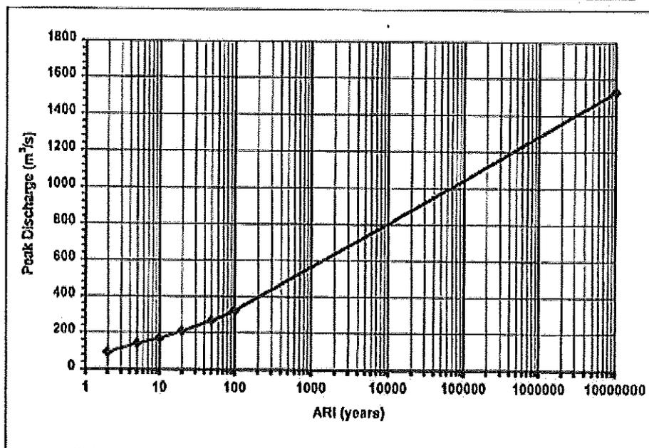
**Figure 9.11: Ultimate Conditions Peak Discharges for Goodna Creek - RAFTS Node JINCG**
