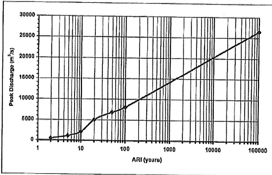
**Figure 7.9: Existing Conditions Design Peak Discharges for the Bremer River - RAFTS Node 1B**
