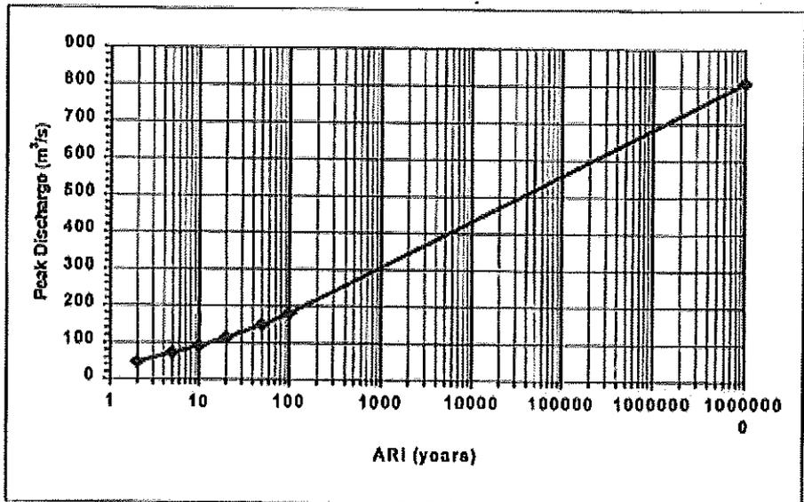
**Figure 7.14: Existing Conditions Design Peak Discharges for Mihi Creek - RAFTS Node MH-OUT**
