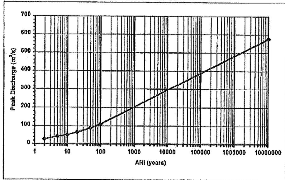
**Figure 9.8: Ultimate Conditions Peak Discharges for Sandy Creek (Chuwar) – RAFTS Node SC-OUT**
