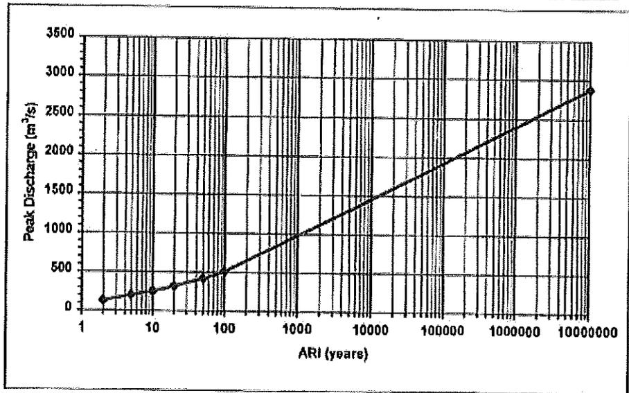
**Figure 9.13: Ultimate Conditions Peak Discharges for Sandy Creek (Camira) - RAFTS Node JIN6J**
