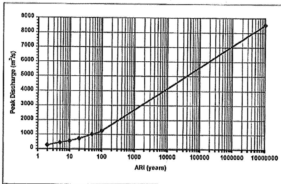
**Figure 9.5: Ultimate Conditions Peak Discharges for Deebing Creek - RAFTS Node DB-OUT**
