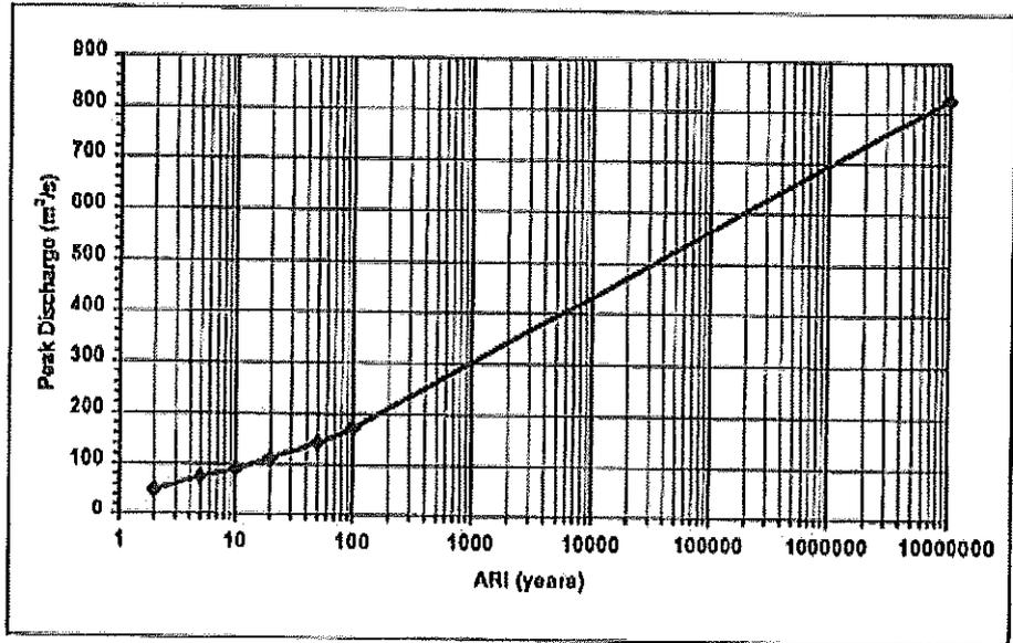
**Figure 9.12: Ultimate Conditions Peak Discharges for Woogaroo Creek - RAFTS Node JIN3M**
