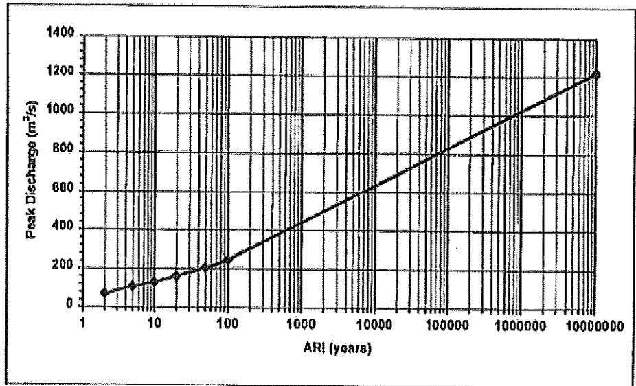
**Figure 9.6: Ultimate Conditions Peak Discharges for Ironpot Creek - RAFTS Node IP-OUT**
