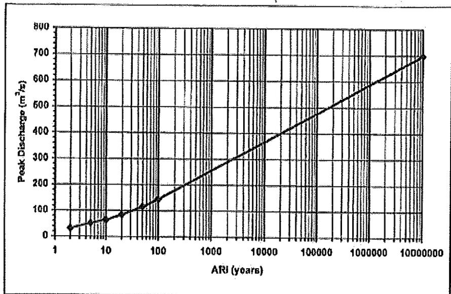
**Figure 7.16: Existing Conditions Design Peak Discharges for Bundamba Creek – RAFTS Node BUND18**
