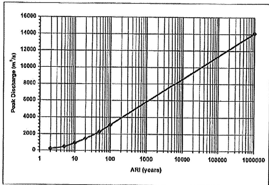
**Figure 9.4: Ultimate Conditions Peak Discharges for Purga Creek – RAFTS Node 6F**
