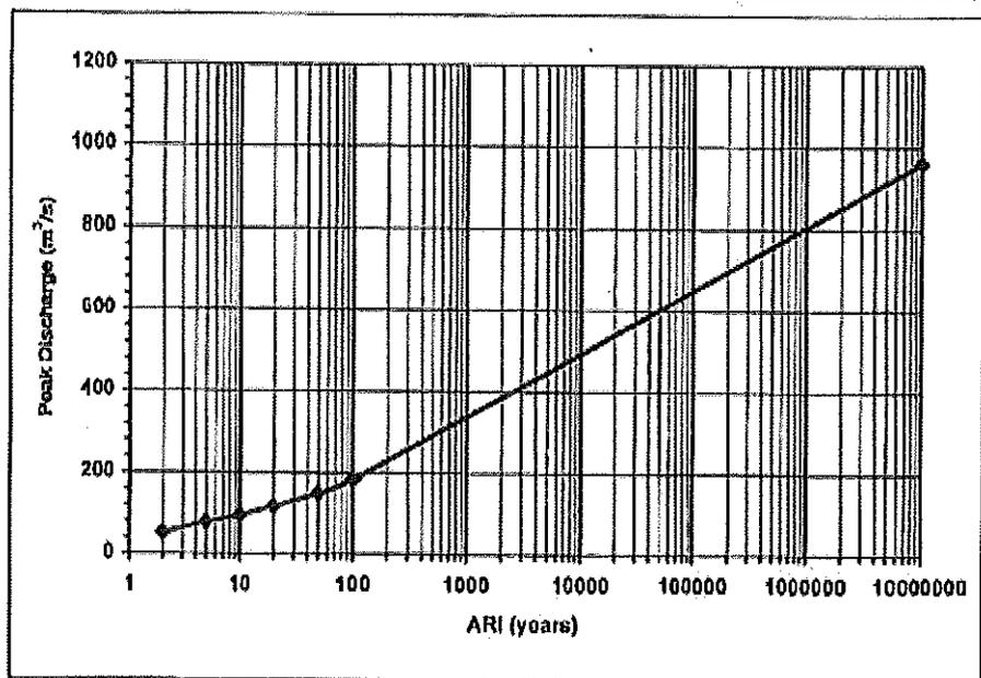
**Figure 9.7: Ultimate Conditions Peak Discharges for Mlhl Creek – RAFTS Node MH-OUT**
