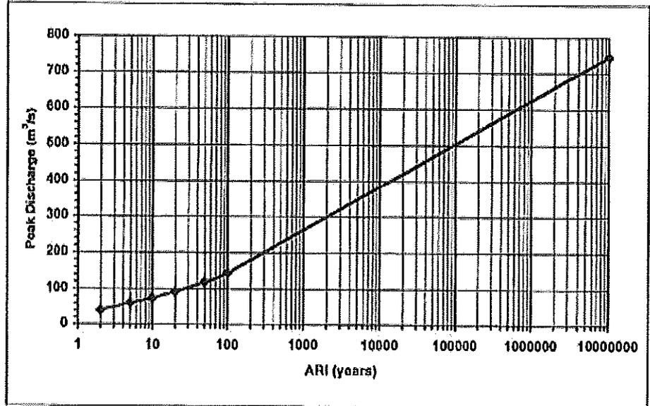
**Figure 7.19: Existing Conditions Design Peak Discharges for Woogaroo Creek – RAFTS Node JIN3M**
