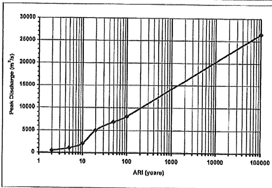
**Figure 9.2: Ultimate Conditions Peak Discharges for the Bremer River – RAFTS Node 1B**
