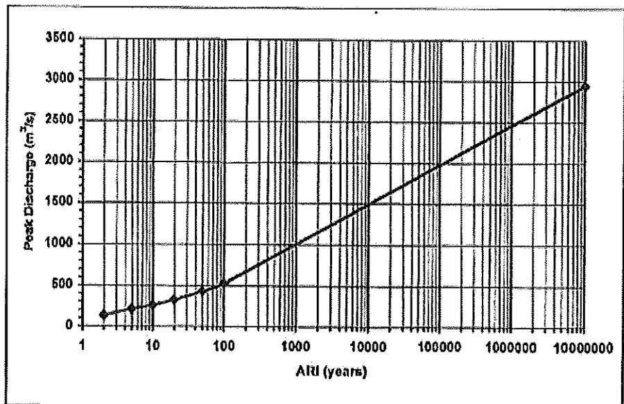
**Figure 7.20: Existing Conditions Design Peak Discharges for Sandy Creek (Camira) - RAFTS Node JIN6J**
