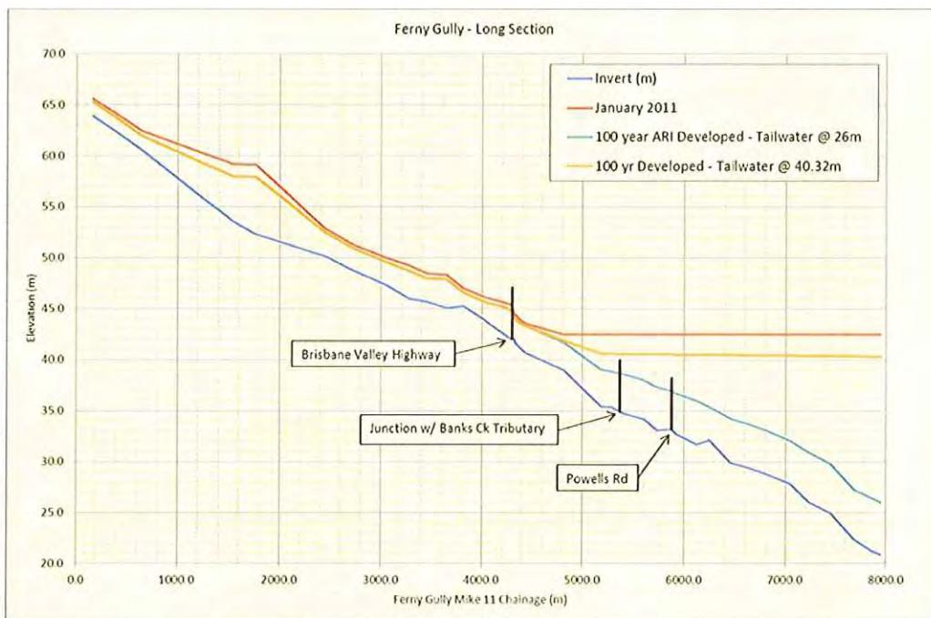
**Figure 5.4 Ferny Gully Water Surface Profiles**
