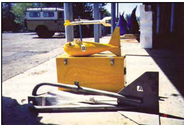
Figure C9.8 Helley-Smith bedload sampler (labelled A) and P 61 suspended sediment sampler (labelled B)
