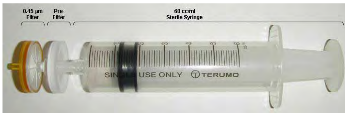
Figure 3.5 Pressure filtration equipment
