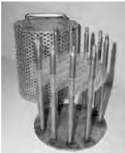
Figure C2 Housing and components of an SPMD passive sampler. The protective cage covers the absorbent strip during deployment
