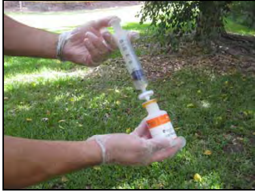
Figure C10.3 Attaching the pre-filter (a) and filter (b) to the syringe and filtering sample into bottle 'E' (c)
