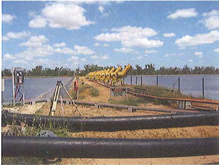
Moranbah North Coal Mine Misters on the Dam wall between two of their dams (1 & 2). Units were not working at time of visit due to unfavourable weather conditions.
