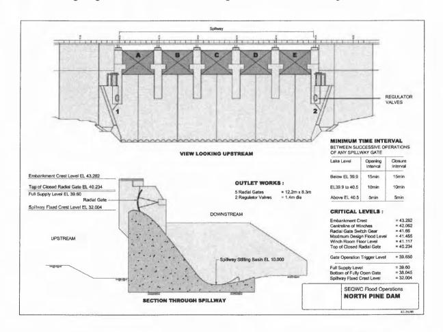
Gate operating sequences are conducted according to target minimum intervals.
