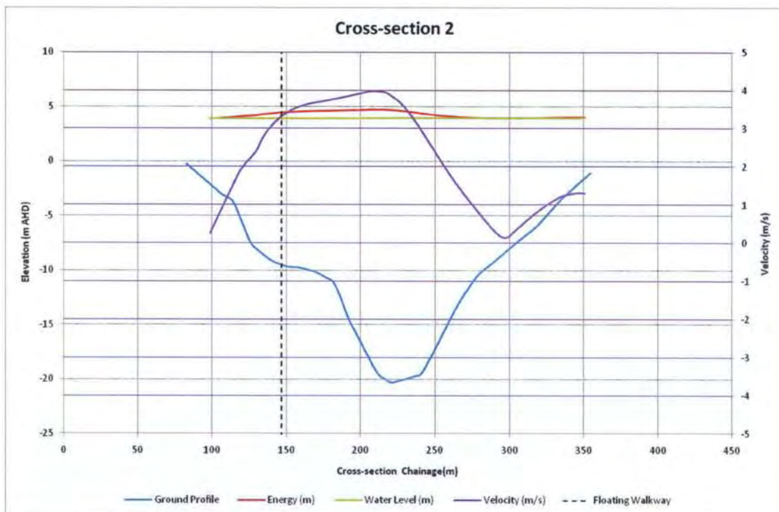
Figure 7: Cross-section Showing Lateral Distributions of Bathymetry, Energy Level, Water level, Velocity, and the Location of the Floating Riverwalk at Chainage 650m
