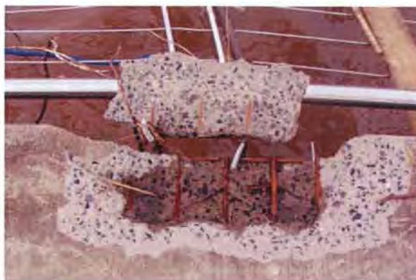
Figure 11 Typical Base Plate Bolt Group Failure Due to Debris Impact
